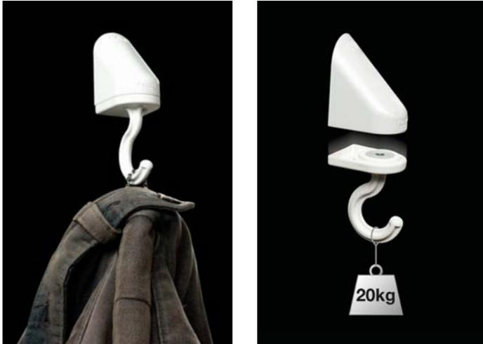
Developed in response to repeated requests from hospital staff, the Kestrel coat hook is the answer to what seemed an intractable problem. A hook was needed that was as strong as a standard coat hook in normal use, yet would give NO point of ligature. The Kestrel coat hook is in two parts which perfectly complement each other, with the hook simply parting from its bracket under abnormal load.
