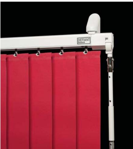
**KVL64 Premium headrail** with wheeled carrier trucks and crank mono control. Optional detachable crank. 127 or 89mm louvres.
